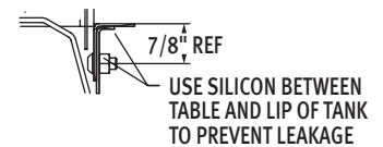
Sectional View Showing Table Connections
