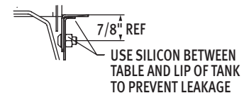
Sectional View Showing Table Connections
