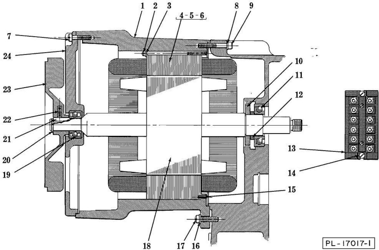
**MOTOR UNIT (3 PH. — DUAL VOLTAGE)**
