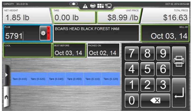
**NOTE:** The Tare Grid, shown above in the dynamic content area, is a feature that can be configured by the supervisor or operator. To change COOL: TOUCH the COOL field. You should now see the *COOL Window*.
