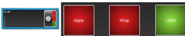
The L in the Operation Mode area will change to green and the PLU# area will be black. Place the product on the wrapper scale. A label will print automatically when a stable weight has been sensed by the scale. The label will not be applied to the product. Manually remove the label from the printer and apply to the product.
