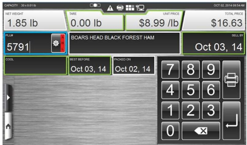
To change Field values: TOUCH the field and TYPE the change on the Keypad. TOUCH Enter. The value change will be displayed in the field. This applies to Unit Price, PLU#, and By Count on the Center Operator Screen. This applies to Shelf Life (Hours), Product Life (Hours), Primary Label, and Additional Labels IDs on the Right Operator Screen.
