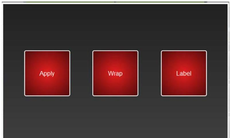
To set the system to automatically wrap the product and print and apply a label: TOUCH the Apply, Wrap, and Label buttons until the buttons are green. TOUCH anywhere outside the Operation Mode Setup Screen to exit.
