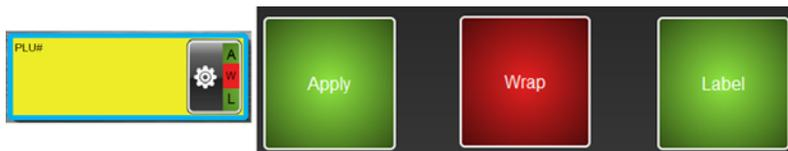
The A & L in the Operation Mode area will change to green and the PLU# area will be yellow. Place the prepackaged product on the wrapper scale. A label will print automatically when a stable weight has been sensed by the scale. The product will travel through the wrapper and the label will be applied. The product will not be wrapped.
