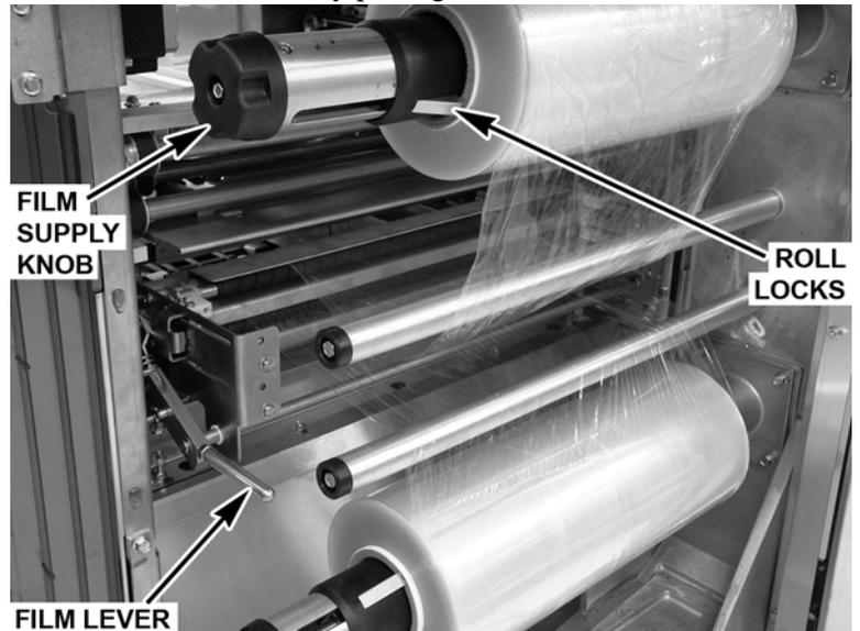
4. Turn film supply knob counterclockwise until roll locks are open 1 to 2 inches wider than the roll width.
