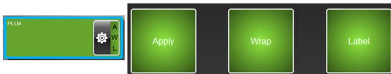
The A, W, & L in the Operation Mode area will change to green and the PLU# area will be green. A product is placed on the wrapper scale. The product will run through the wrapper and will be wrapped. A label will be printed when a stable weight has been sensed by the scale. The label will be applied to the product as the product emerges from the wrapper.
